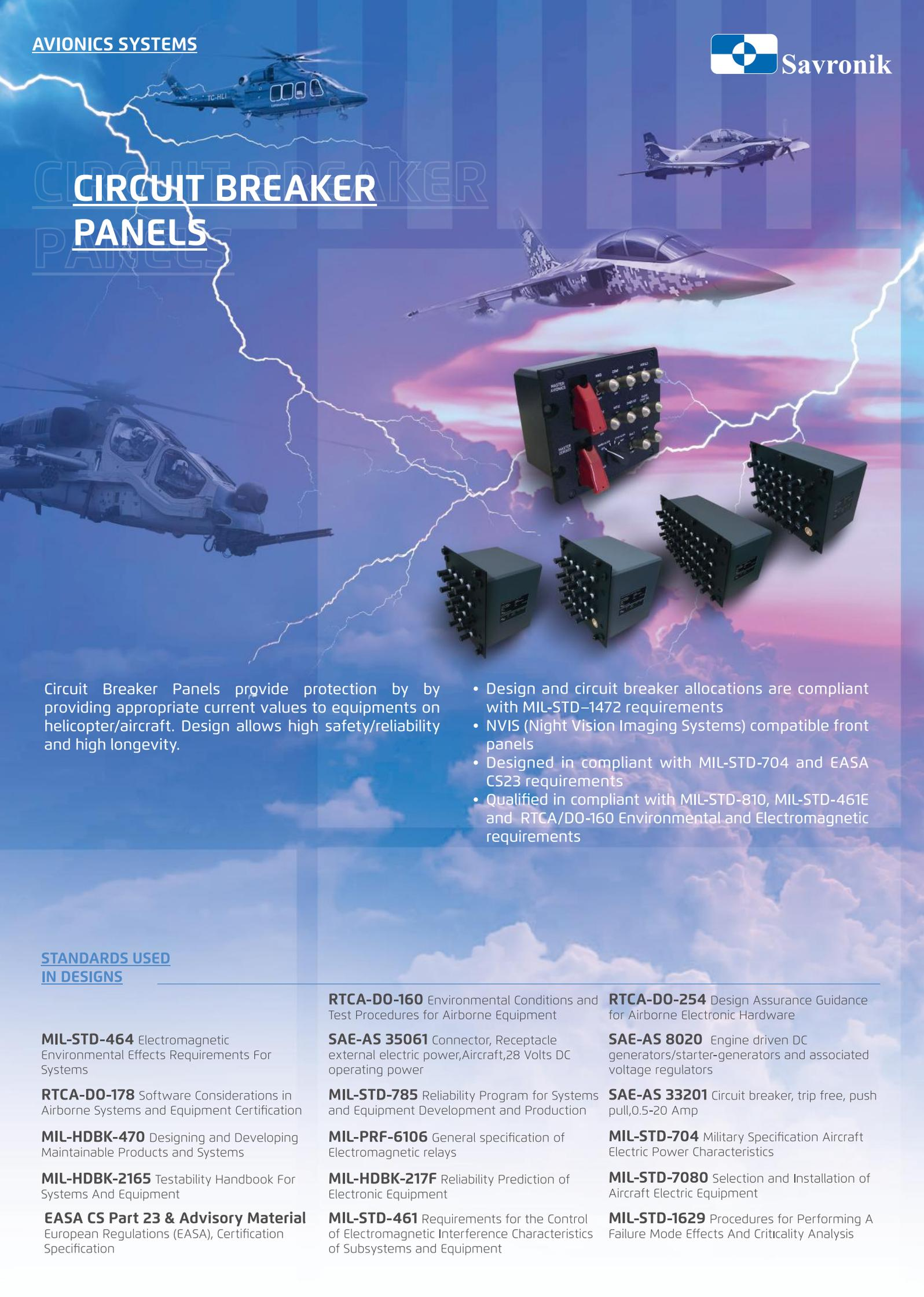
Circuit Breaker Panels provide protection by providing appropriate current values to equipments on helicopter/aircraft. Design allows high safety/reliability and high longevity.
